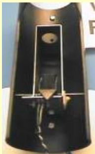
If this fails the plug in the bottom of the rain water collector can be removed to allow access.
