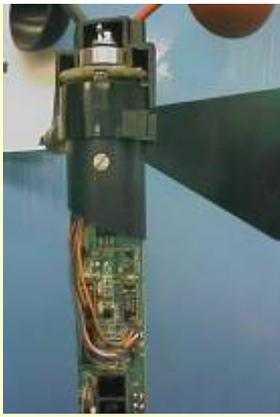
Without special equipment it is not possible to test the light sensor. This is an Infrared collector whose output is used to detect sunrise/set by a change in the IR radiation above or below a threshold level.
