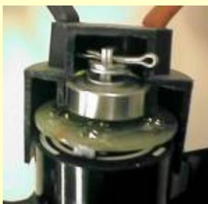
If the Wind-vane and Anemometer require attention you can push the anemometer off its bearings by pushing upwards against it with your thumbs. This will expose the printed circuit board, and show the top of the wind-vane. The printed white circles on the top of the wind-vane can be cleaned using a cotton bud. Ensure that it is fully seated on its bearing, leaving a few millimetres between the painted surface and the sensors on the underside of the circuit board.
